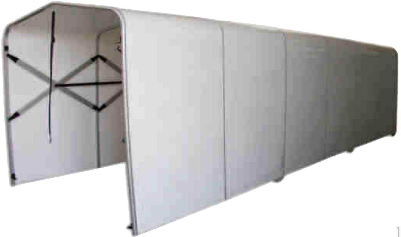
Constructed on an anodised aluminium structure, with a 43 x 35 mm extruded profile for the arcs, which allows for the canvas panels between them to be replaced individually by the client himself if damaged, therefore avoiding the tunnel having to be sent to the manufacturer.
